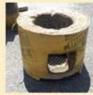
Molded combustion chamber incorporating grate and ash tray
