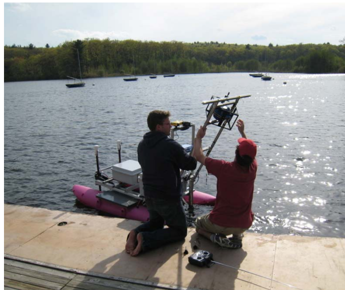
Image 2: Craft with hydrophone and source in launch/transport position.
