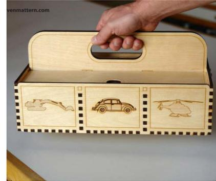
This joint can be used to create partitions in a box. Note that in the toolbox by Steven Mattern, finger joints were used on the outside edges while mortise and tenon joint were used to create the non-corner partitions between the helicopter, car, and backhoe.
