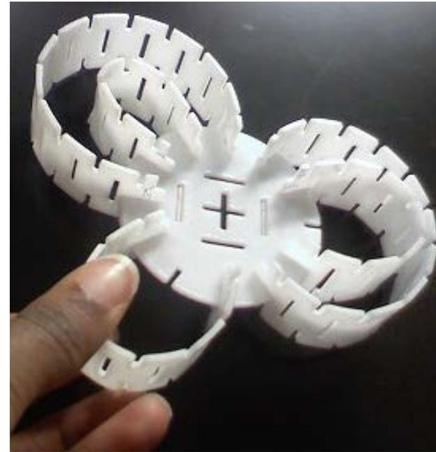
To create a rougher finish, this maker changed the frequency of her laser cutter to create a more jagged surface that could grab hold of a surface.
