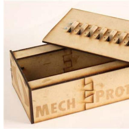
This use of a dovetail joint is mostly aesthetic, but it demonstrates how a dovetail could be used to join two pieces of flat material. It could be especially useful when making something that is larger than the capacity of the laser cutter (by Holzgrafe and O'Toole).
