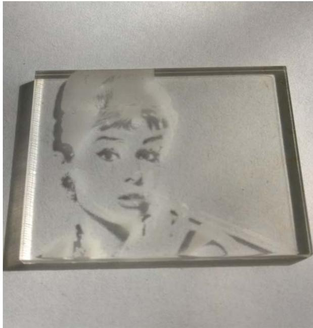
Engraving acrylic on the underside of the material allows the image to be seen through the thickness of the piece. Mirror your graphic in your cut file to produce the correct final engraving.
