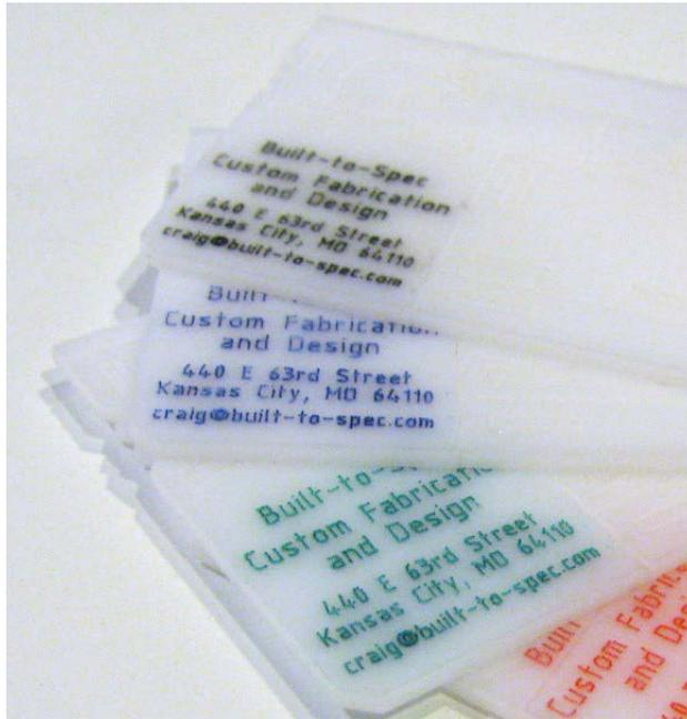
When you raster white Delrin, the rastered image is white. But you can create “synthetic” contrast. After rastering a design, blot the area with a dry erase marker and let it wick into the Delrin. Once it seeps long enough, wipe away the excess to reveal your design. Make sure to do some prototyping with this technique.
