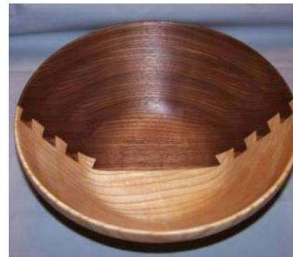
The bowl pictured here is made from laminated scrap wood and uses the dovetail as an aesthetically pleasing way of joining individual pieces.
