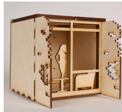
Mortise and Tenon Joints hold the front panels of this box in place (Morse and Sutantio).
