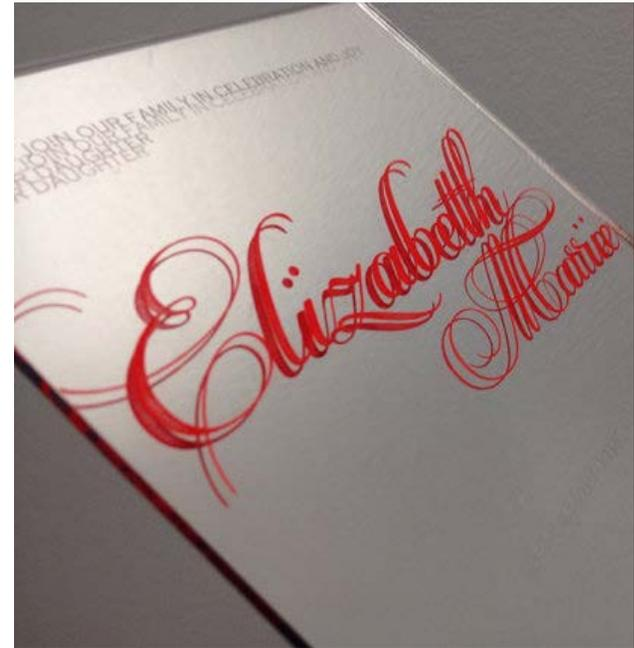
Single surface mirrored acrylics come with a reflective side and an opaque backing on the opposite surface. When engraving mirrored acrylic, a double image will occur if engraving on the reflective surface (you can engrave on the back side instead). When vector cutting mirrored acrylic, cut with the mirrored surface up and don't worry about the laser reflecting off of the material because it will be absorbed by the acrylic first.
