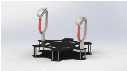
Figure 2. CAD render of hanging landing gear.
