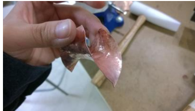
(L) Synclast rectangle. (2) Anticlast hyperbolic paraboloid extension.
