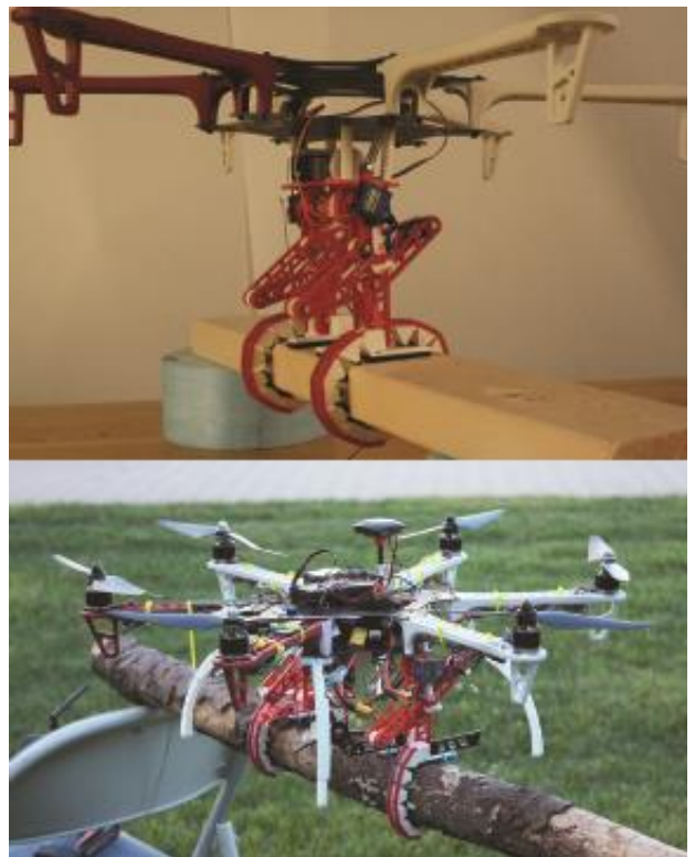
Fig. 3 A hexacopter frame and a flight-ready hexacopter stably perch on a wood board and on a tree branch. The weight of the air vehicle tensions cable tendons which curl the feet and grasp.
