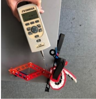
Fig. 7 Experimental setup for tension measurements. Gage value is halved to account for the two tendon loop on hook.
