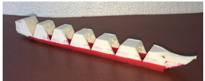
Fig. 2 A six-segment, compliant foot fabricated by 3D printing a flexible thermal-plastic (red) and stiff ABS (white). Length: 13 cm. Segment heights: 0.9-1.7cm.
