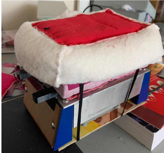
Fig. 3. Guarded Hot plate setup
