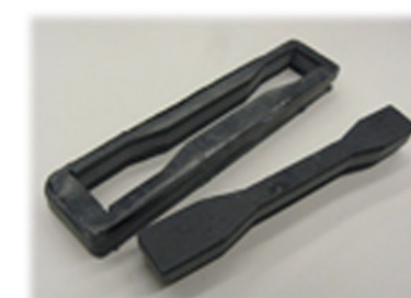
Some of our samples were water jet cut into dogbone shapes for tension test samples.
