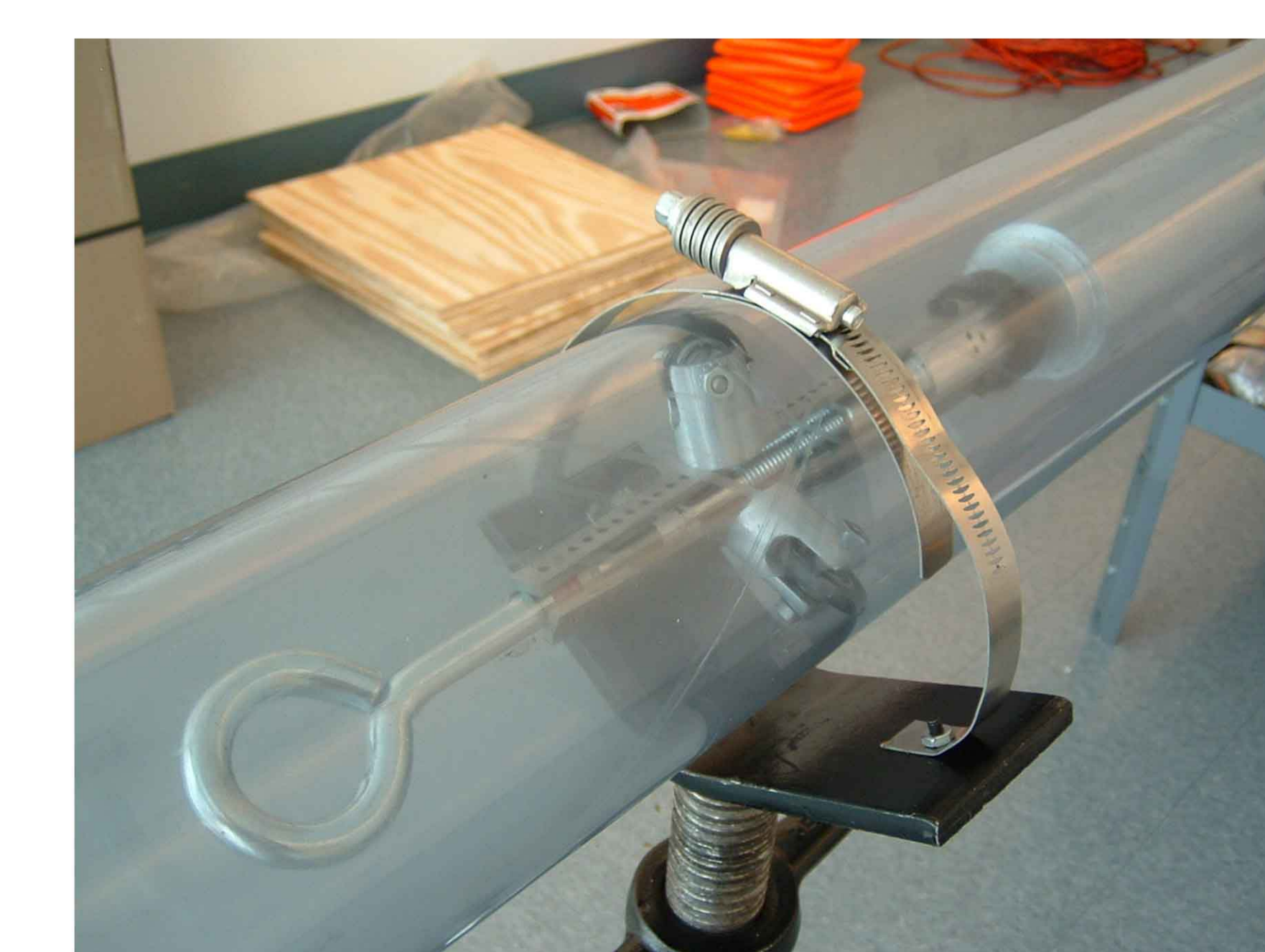
▲ In this picture of the test setup, the wheels are angled at 45° with respect to the test tube.
