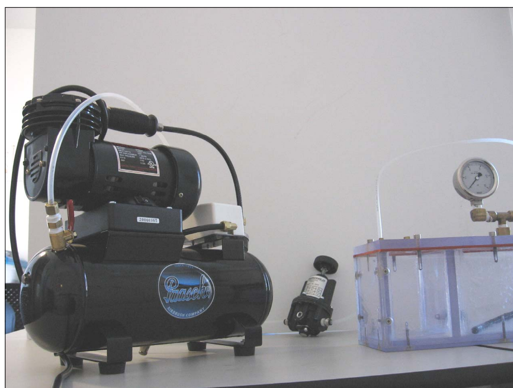
Test stand and catheters used for seal testing
