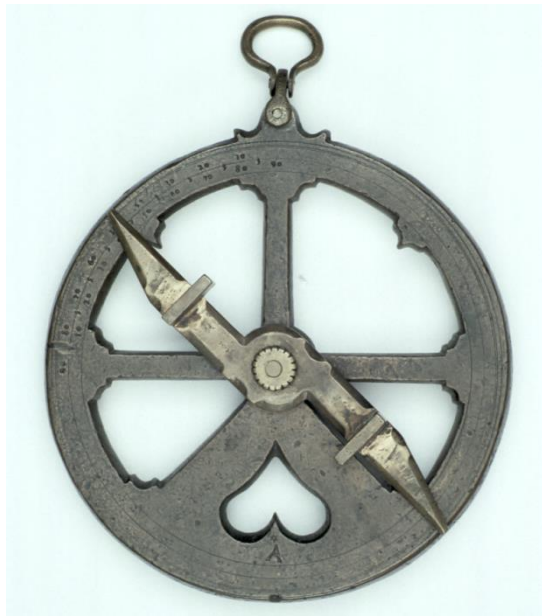
Figure 6: Mariner's Astrolabe- This Spanish astrolabe, dated to around 1600, was found drowned in the Gulf of Mexico and currently resides in the Museum of History of Science in Oxford, UK 16 . Note the lack of rete or plates typical of land astrolabes; this instrument was purely a pointing device, not a map of the heavens.
