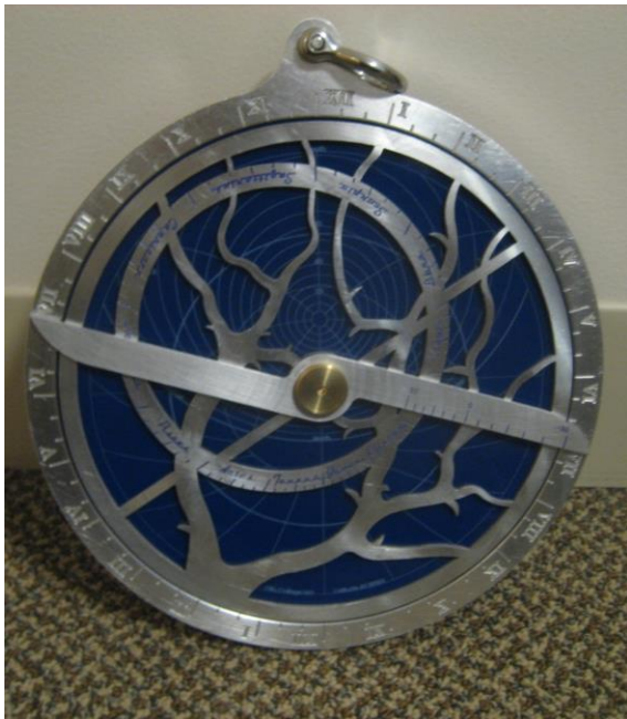
Figure 7: My Astrolabe – The astrolabe is approximately 8.5 inches across, making it on the larger range for an astrolabe. Typical time measurements are accurate to within 5 minutes.
