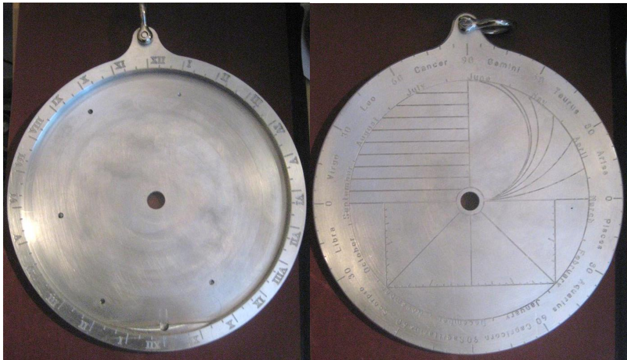
Figure 13 – Front and back of the Mater, Final Part
